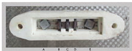
Fig. 12.11: The Simple spark gap device diverts lightning strike to the ground (earth)
