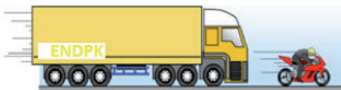
Fig. 8.3: The Kinetic energy of a moving body depends on its mass and velocity
