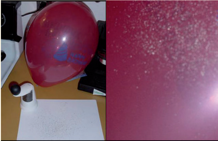
Fig.12. 20: Materials required for the balloon model electrostatic precipitator. Close-up of pepper grains on the balloon surface.
